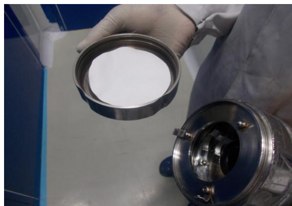
3. Air Sampler having whatman filter of 0.4 micron.
