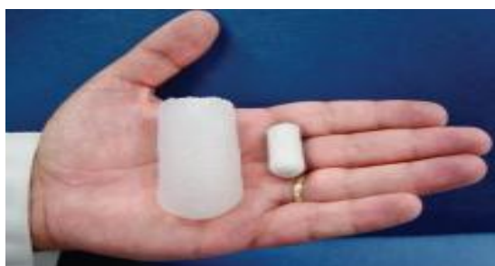
Figure 3: A Superporous Hydrogel in its Dry (Right) and Water-swollen (Left) State.
