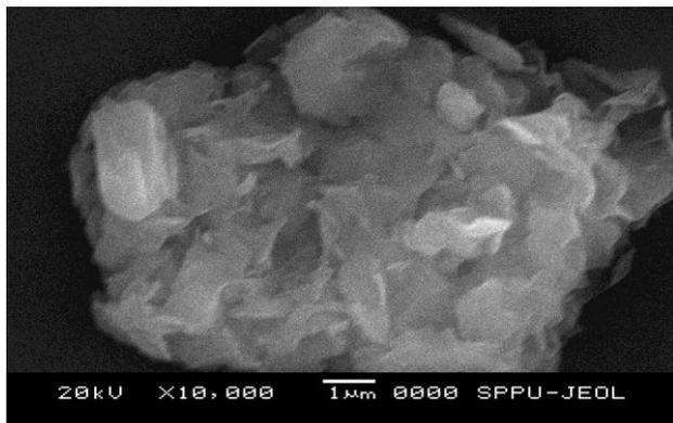
Figure 5: SEM of MMT-ICZ complex ( $\times 10,000$ ).
