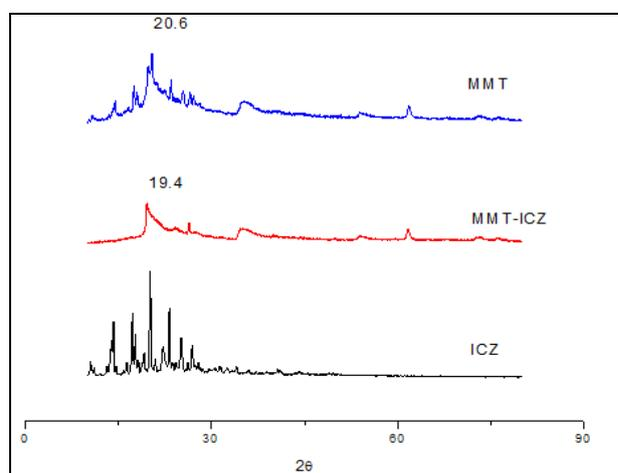
Figure 3: PXRD patterns of ICZ, MMT-ICZ and MMT.
