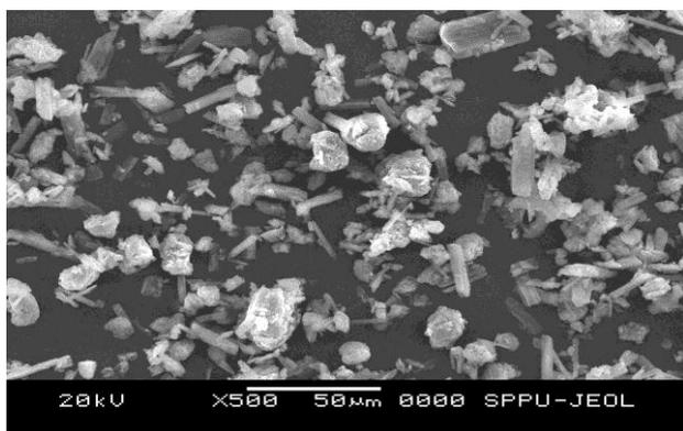
Figure 5: SEM of MMT-ICZ complex ( $\times 500$ ).
