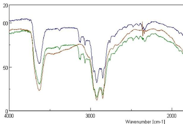
Figure 4: FTIR spectra of ICZ MMT-ICZ, MMT.
