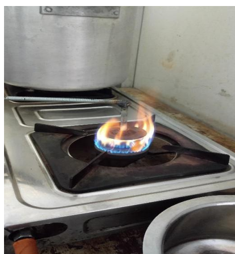
Step 4: Iron rod heated on burner.
